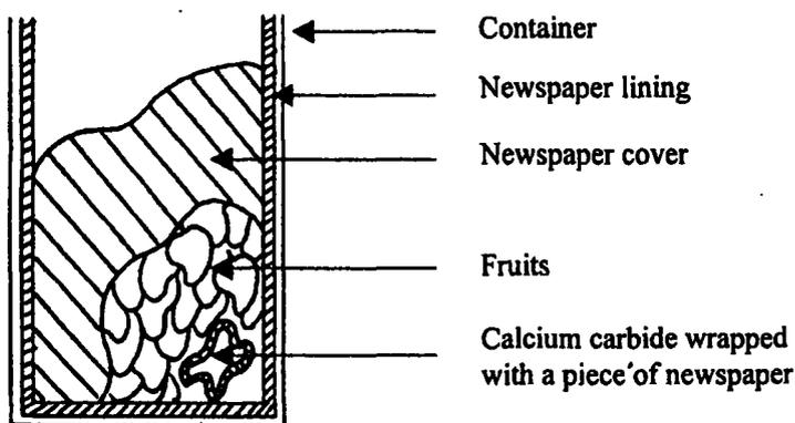
**Figure 1.** A cross section of a container of fruits treated with calcium carbide.
